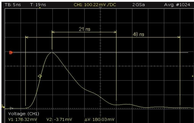
The figure shows a 10% recovery time for the APD tile of 21 ns, which is equivalent to below 50 ns recovery time to 1% and thus well within the total pulse length.
