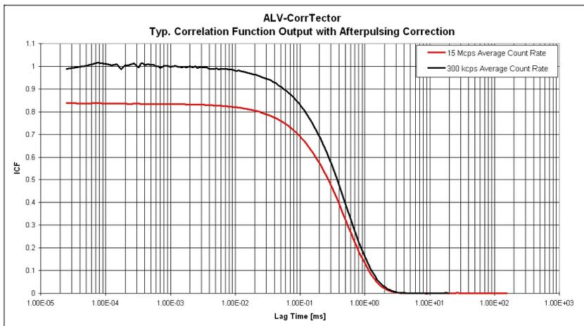
Low (300 kcps) and high (15 Mcps) average count rate correlation functions shown with afterpulsing correction applied.
